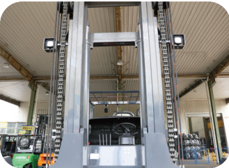
Wide field of view mast improves the safety of stacking operations.
