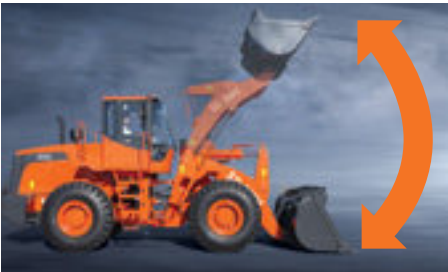
Arm Raise Kick-out and Return to dig function : reduce the intensity of your work and improve working efficiency.
