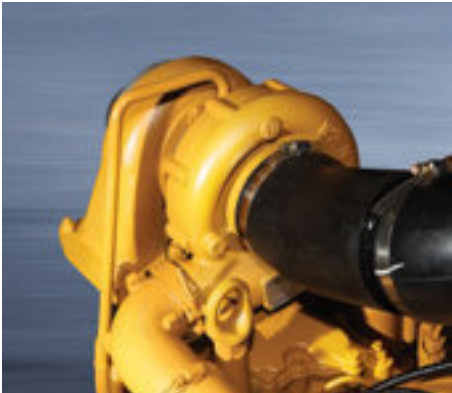
Use exhaust turbine to increase pressure, therefore, torque reserve is large and the fuel consumption and engine oil consumption are low with good altitude adaptability which meet the emission standards of Tier II. The low speed of 2,000rpm + perfect power matching+dual pump confluence technology make DISD loaders more fuel efficient compared to competing enterprises under the same working condition.
