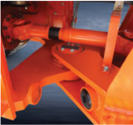
Hinge Limit DISD loader adopts a new part - the nylon hinge limit block. It has stronger durability, no noise caused by impact and reduces the driver's fatigue.
