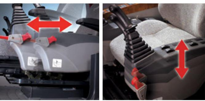
Comfortable 2-stage sliding seat Control stand (Telescopic Function)
