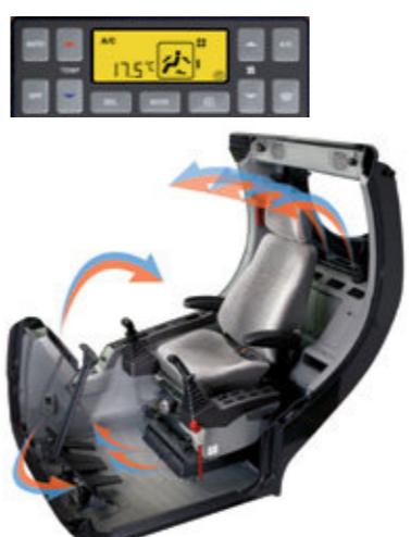
The high performance air conditioning provides an air flow which is adjusted and electronically controlled for the conditions. Five operating modes enable even the most demanding operator to be satisfied.
